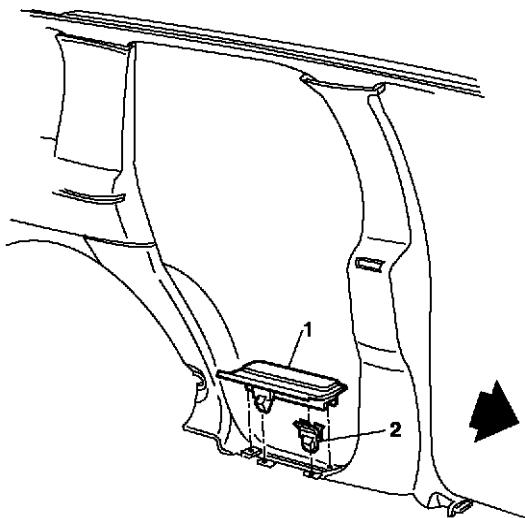
Install the door sill trim plate (1) onto the vehicle.
