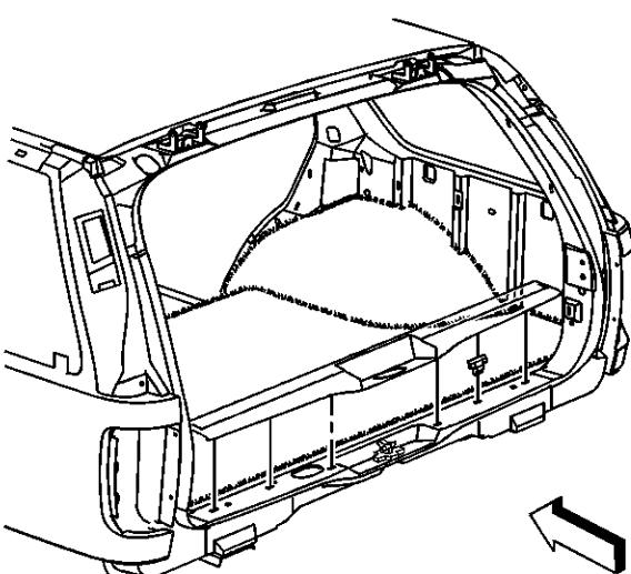
Use the [J38778](#) in order to remove the door sill trim plate from the vehicle.
