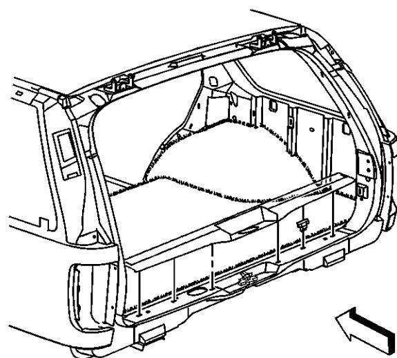
Install the door sill trim plate to the vehicle. Align the retainers along the door sill and press into place.
